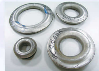
Welded Tube Extension Test
