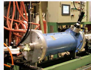
Heating Coil (with Infrared Temp. Detector)
