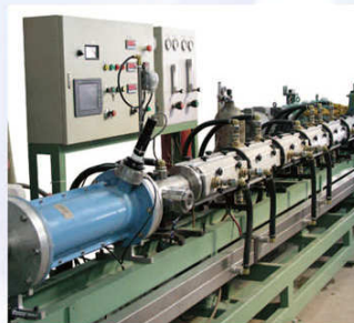
In-line Bright Annealing Cooling Section
